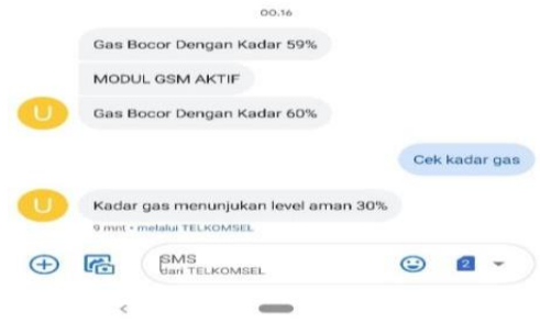
Figure 13. Sms Display Sent by the Device When a Gas Leaks Detected
